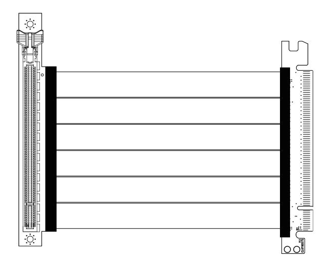
200mm PCI-E 3.0 Extend cable for VGA card
