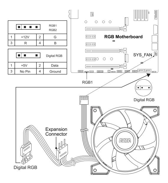
The addressable RGB fans can connect directly to the 5V addressable RGB headers of compatible motherboards, such as those from MSI™, ASUS™, Gigabyte™ and AsRock™.
