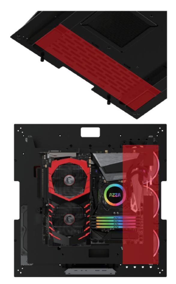
■ Supports up to 120mm fans x 3 / 240 / 360mm water radiator
