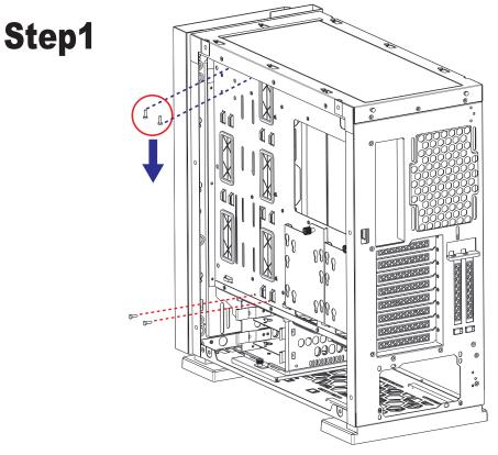
•Remove the screws from the front cable management bar.
