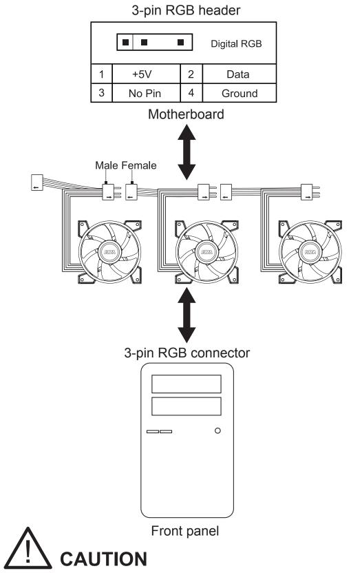
The addressable RGB fan has a 3-pin connector (4 holes). Please ensure that you are connecting the 3-pin connector on the fan to the 3-pin RGB header on the motherboard or RF Remote connector. Do not plug it into the 4-pin header, as the incompatible voltage will fry the fan. The 3-pin connector on the fan still has 4 holes, but the 4th hole is intentionally blocked for this reason, so please do not try to force it!
