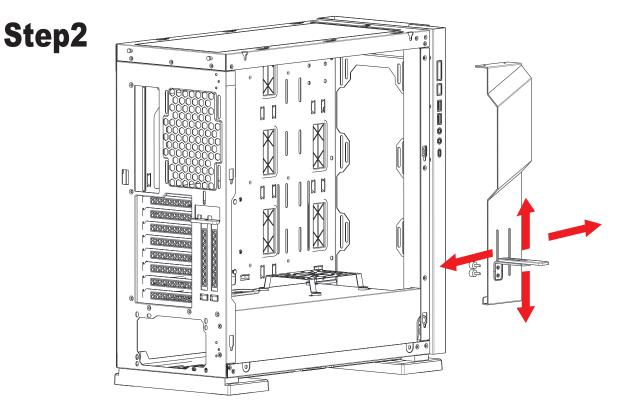
•Video card holder can be adjusted with the thumb screws.
