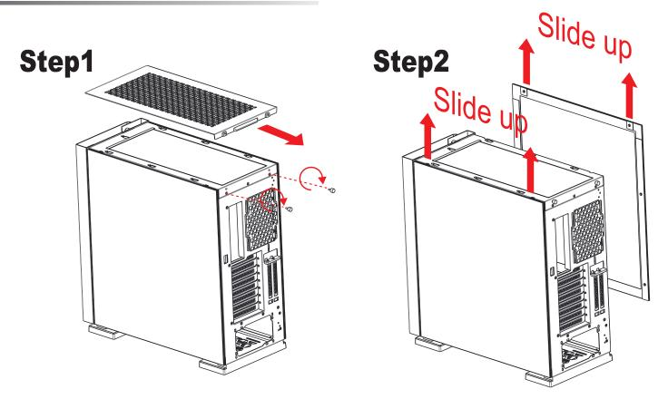
Removing the bottom dust filter
