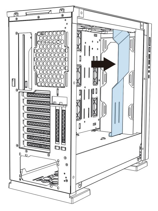
To install the E-ATX(<270mm) motherboard, please take out the cable management bar.
